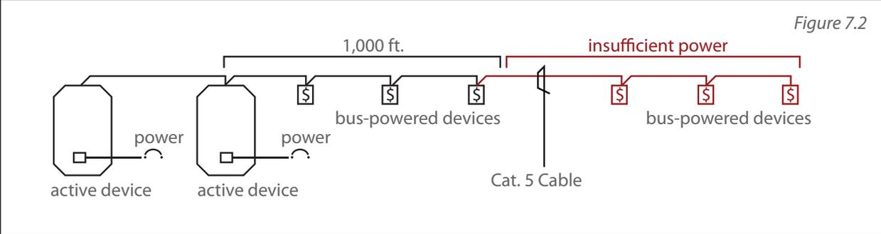
Multiple panels do not increase the distance. For the above scenario, the correct solution would be to route the Cat. 5 properly so as to spread the active devices out. This is shown below:
