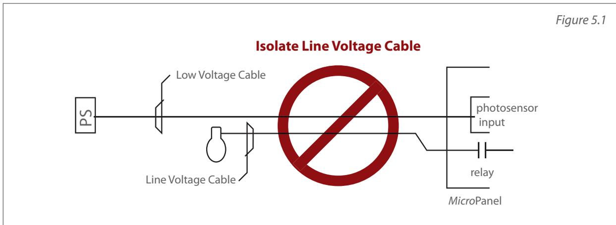
*Low voltage cabling must avoid EMF or RF from ballasts or other “noisy” loads. EMF or RF interference can create an unstable bus and can eventually ruin digital devices.*
