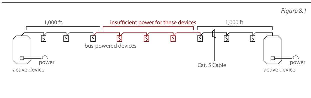
*The Bus Booster adds current to the bus; it does not amplify the digital signal.*
